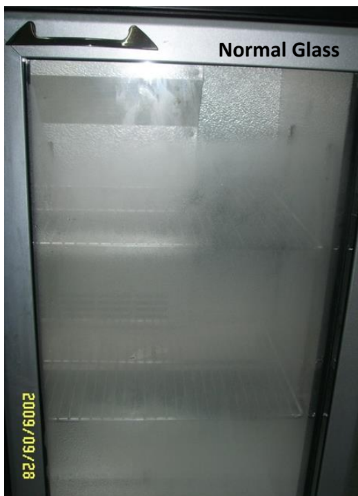
Below shows 70% humidity with Normal Glass on left and LOW E Glass on right.
